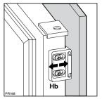
Fix cover (Hd) on guide (Hb) until it clips into place.
